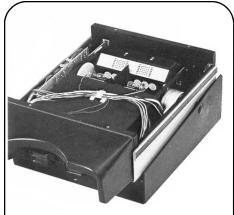
Target drum and illumination lamps are readily accessible by removing the top cover of the case. The drum accommodates eight permanently-mounted stereoscopic tests that may be removed if required under special circumstances. (Instructions for re-installation are presented on page 14).
